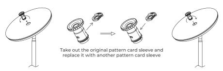
Rotate counterclockwise to take out the projection assembly
